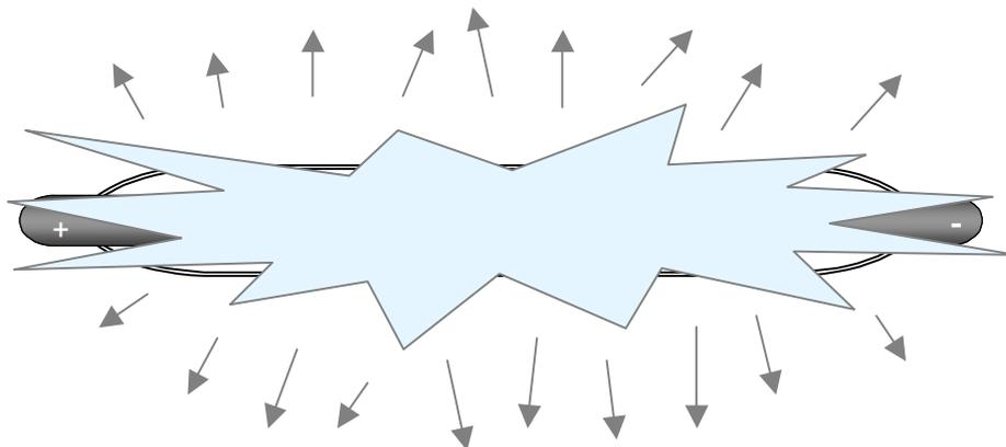
During a pulse the arc expands emitting an intense pulse of light. Unlike a laser an IPL Flashlamp produces an intense pulse of white light, that is light with many wavelengths. The light is not coherent and is emitted in all directions.
